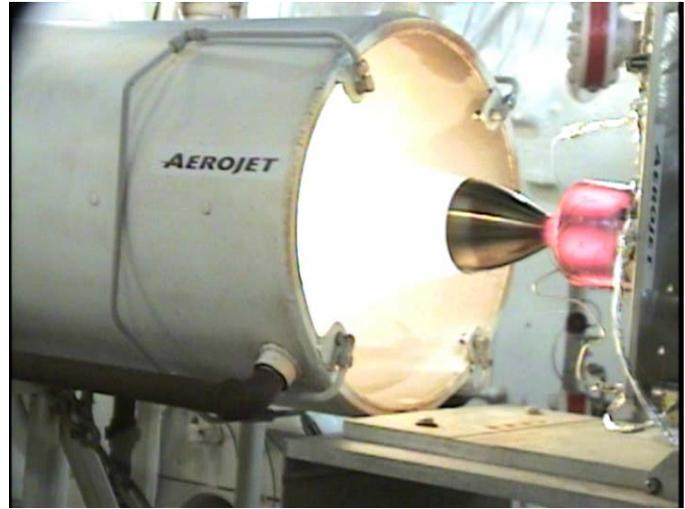
**Figure 11—MLE Engine Demonstrates Pulse Mode Operation at Sea Level**
