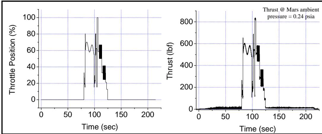
**Figure 6. Qualification Test Duty Cycle and Thrust Response (MDC 2)**
