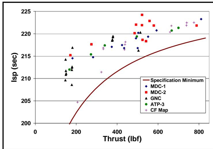
**Figure 7. Qualification Test Specific Impulse vs. Thrust**
