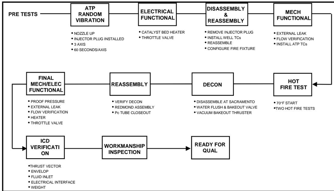
**Figure 2. Acceptance Test Plan**
