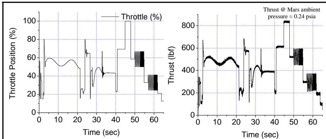
Figure 5. Qualification Test Duty Cycle and Thrust Response (MDC 1)
