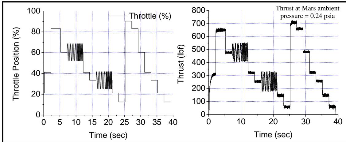
**Figure 3. Acceptance Test Duty Cycle and Thrust Response (Test ATP-1)**
